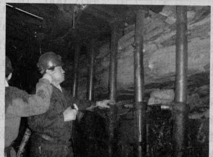
图 3 榆阳煤矿 3 煤上覆岩层冒落特征图 Fig.3 The features of fall of overlying strata in No.3 Yuyang coal mine
