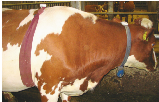
Fig. 4. The tag on a cow's collar and on a cow's back with a special band
