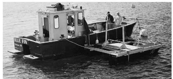
Fig. 3. The data acquisition catamaran alongside the workboat Blue Fin .
