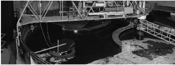
Fig. 3. Elevated view of the setup in the Coriolis rotating tank. The scanning laser head and mirror were fitted inside the gray box fixed to the tank rim with a steel bar. The observation bridge held the actual laser (connected to the laser head below) and computer acquisition equipment, connected to the camera located above the center of the channel below. The channel connected the two large reservoirs and had a removable barrier.
