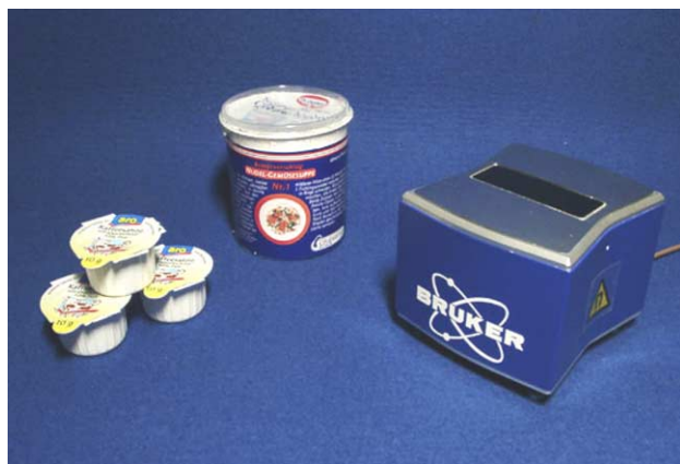
Fig. 7. The Bruker single-sided NMR device called minispec mq-ProFiler, specially designed for industrial needs. Creme samples are shown for comparison of size.
