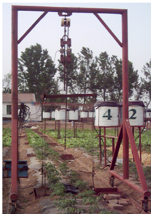
Fig. 2 – A set of weighing lysimeter showing the rail-guided and hoist.
