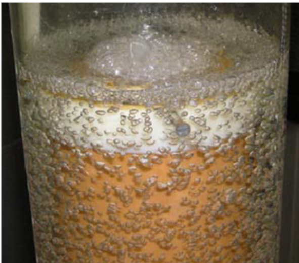
Fig. 5. Bubble flow regimen in the reactor.
