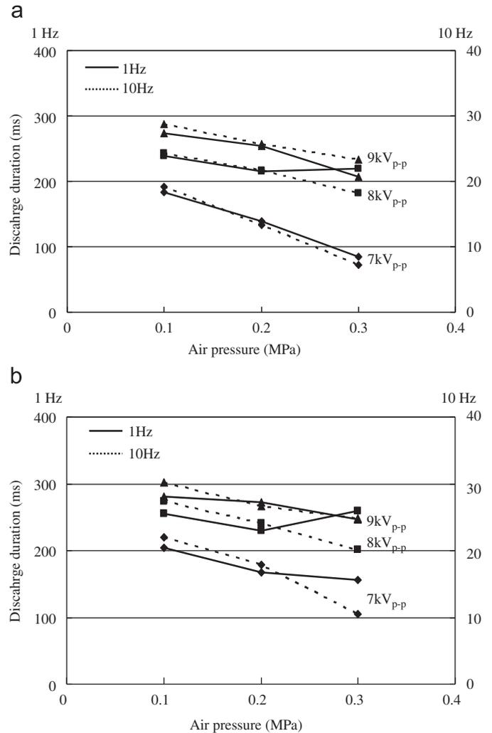
Fig. 6. Dependency of discharge duration on air pressure: (a) positive ion and (b) negative ion.
