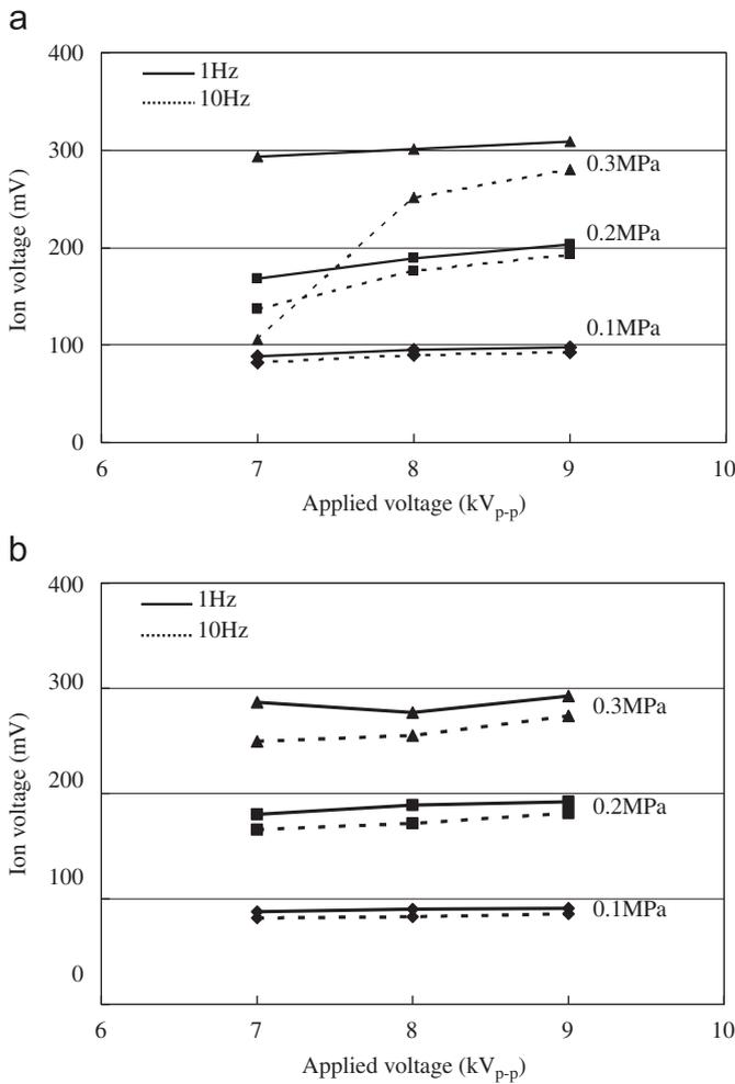
Fig. 3. Dependency of ion voltage on applied voltage. Dividing ion voltage by  $1\text{M}\Omega$  transfers to ion current: (a) positive ion and (b) negative ion.
