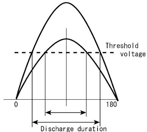
Fig. 8. Schematic illustration of discharge duration with different voltage.
