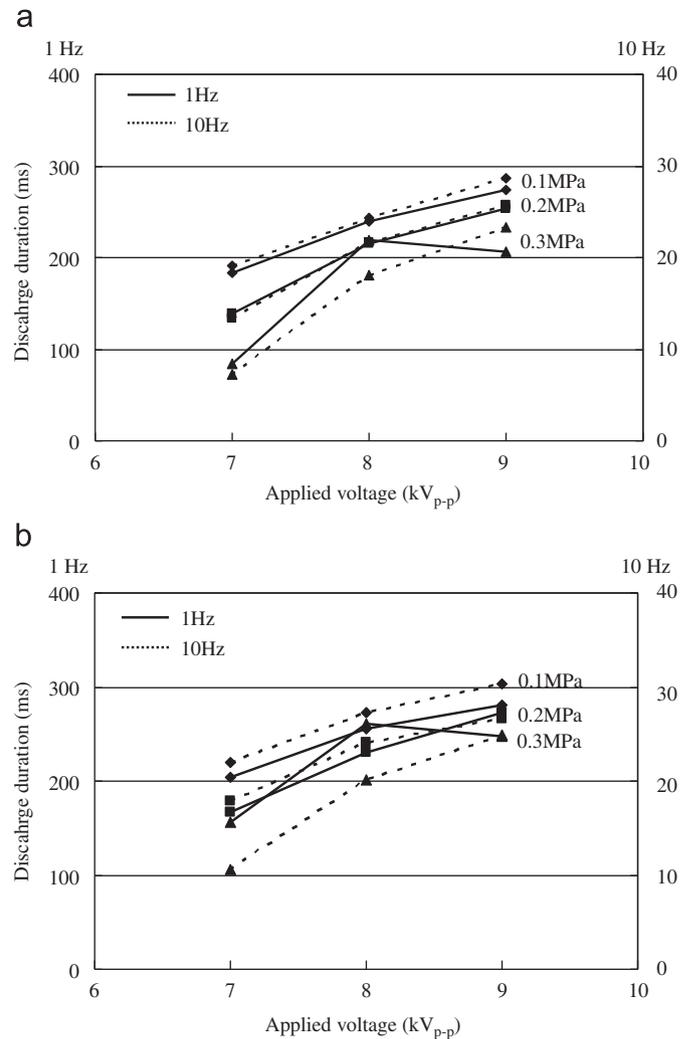
Fig. 4. Dependency of discharge duration on applied voltage: (a) positive ion and (b) negative ion.
