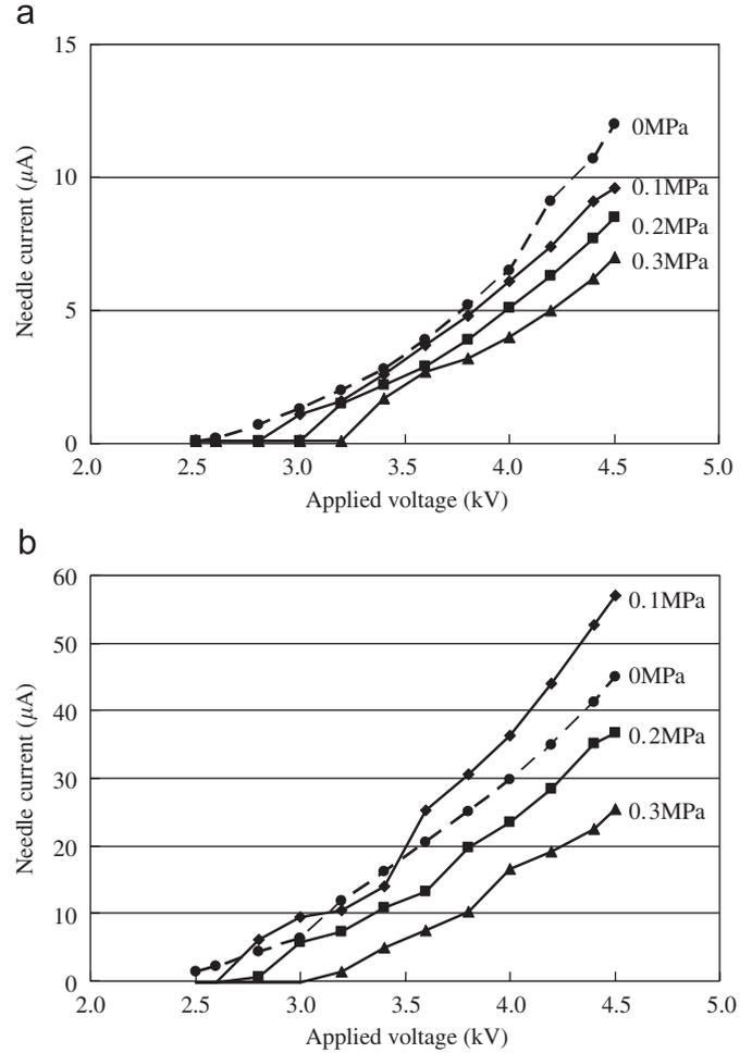
Fig. 11. Dependency of needle current on applied voltage: (a) positive ion and (b) negative ion.
