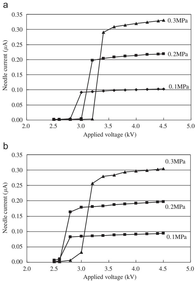
Fig. 12. Dependency of transmitted ion current on applied voltage: (a) positive ion and (b) negative ion.
