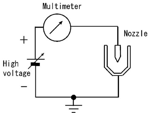
Fig. 10. Ion current measurement with floated state.
