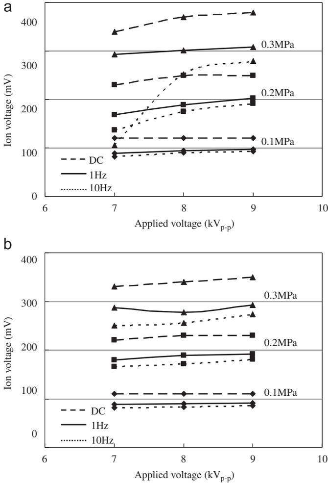
Fig. 9. Dependency of ion voltage on applied voltage. Dividing ion voltage by 1MΩ transfers to ion current: (a) positive ion and (b) negative ion.
