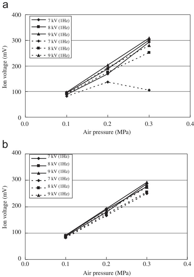
Fig. 5. Dependency of ion voltage on air pressure. Dividing ion voltage by  $1\text{ M}\Omega$  transfers to ion current: (a) positive ion and (b) negative ion.
