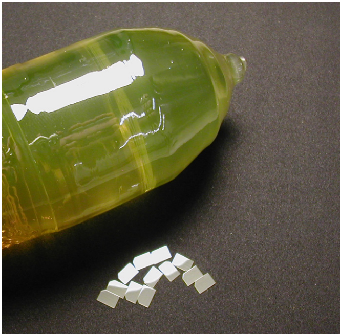
Fig. 1. \text{Al}_2\text{O}_3:\text{C,Mg} crystal and 4 \times 6 \times 0.5 \text{ mm}^3 FNTD.
