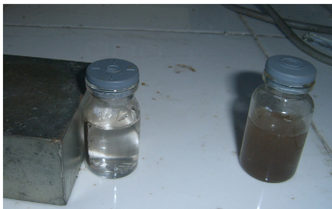
Fig. 8. Photograph showing the stability of the magnetic nanoparticles dispersion (right vial) and the ready capture of the nanoparticles by a magnet (left vial).
