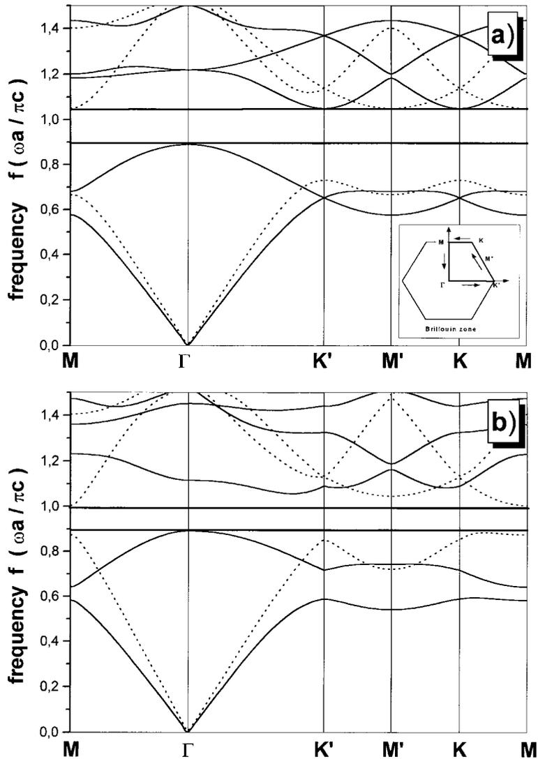
Fig. 2. PBSs for TM- (solid lines) and TE-mode (dotted lines) of a triangular lattice of air pores in Si ( $\epsilon = 11.7$ ),  $r_0/a = 0.468$ ,  $\gamma_e = 0.7945$ , 535 plane waves. (a)  $a_c/b_e = 1$ —circle; and (b)  $a_c/b_e = 0.8$ ,  $\varphi = 0^\circ$  (complete gaps are marked by horizontal lines!).
