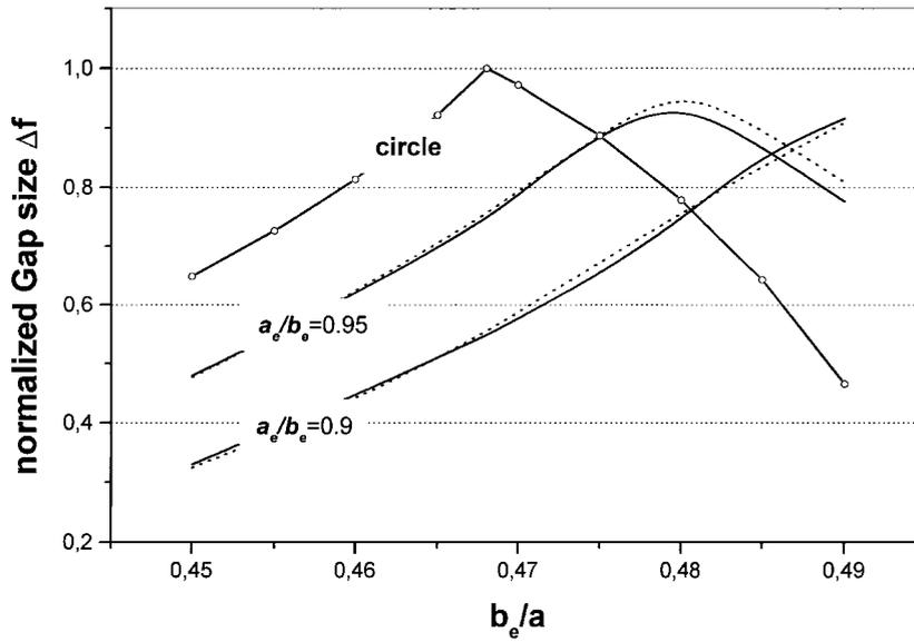
Fig. 3. Complete band gap variations for a triangular lattice of elliptical air holes in Si ( $\epsilon = 11.7$ ),  $b_c$ -axis fix, 535 plane waves.  $a_e/b_e = 0.95$ , 0.9. Angle  $\varphi = 0^\circ$  (solid) and  $\varphi = 30^\circ$  (dotted).
