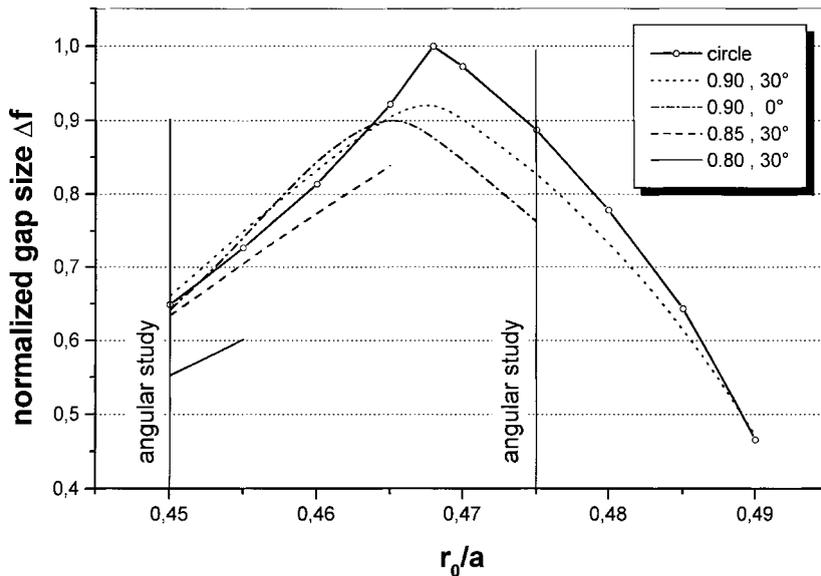
Fig. 4. Complete band gap variations for a triangular lattice of elliptical air holes in Si ( $\epsilon = 11.7$ ), fill factor fix, 535 waves. Values of  $a_e/b_e = [0.8, 1.0]$  and angle  $\varphi$  in the legend.
