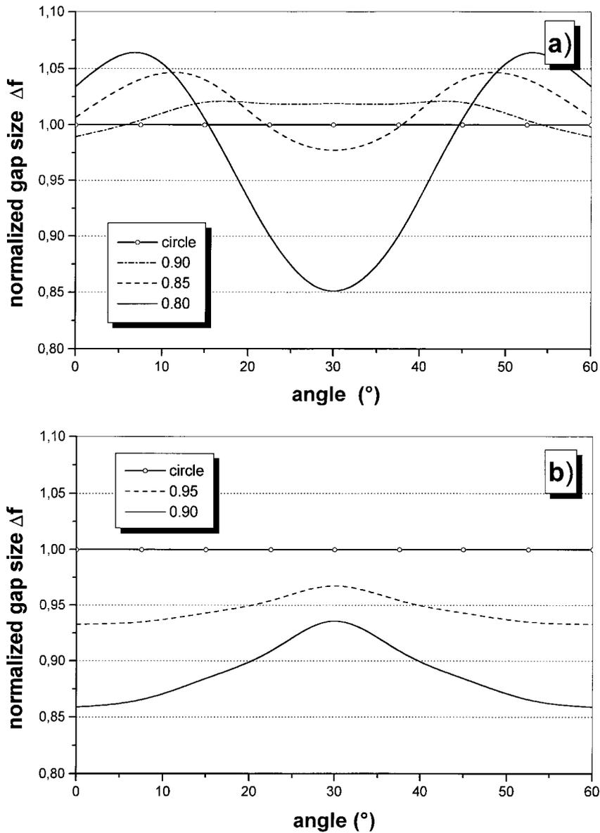
Fig. 5. Angular variations of complete band gaps for a triangular lattice of elliptical air holes in Si ( $\epsilon = 11.7$ ): (a) below ( $r_0/a = 0.450$ ), and (b) above ( $r_0/a = 0.475$ ) the maximum circular pore gap, fill factor fix, 535 waves.
