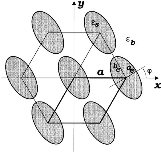
Fig. 1. Model of a PC (triangular lattice of elliptical pores).
