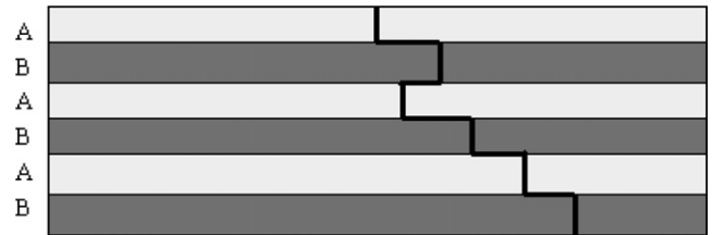
Fig. 6. Crack propagation path of interply composite in low velocity impact.
