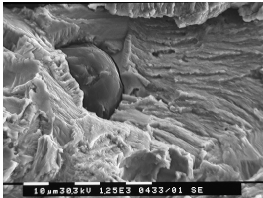
Fig. 14. SEM fracture surface analysis: austempered ductile iron ( R = 0.5 , \Delta K = 10 \text{ MPa } \sqrt{\text{m}} ).
