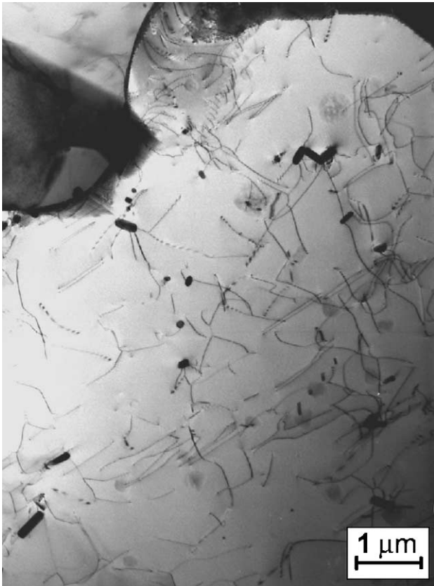
Fig. 3. Structure of the not annealed sample (A) after creep at 600°C.
