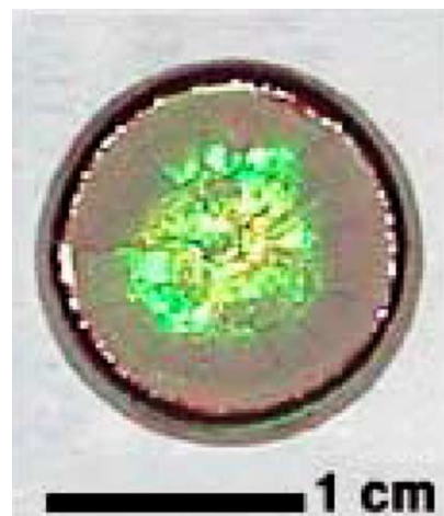
Fig. 2. Photograph showing the opalescence of an ordered macroporous RF aerogel. While the entire monolith is templated, only the center of the material appears opalescent at this angle when illuminated with visible light due to surface curvature. The dark material around the edge of the disk is untemplated RF aerogel.
