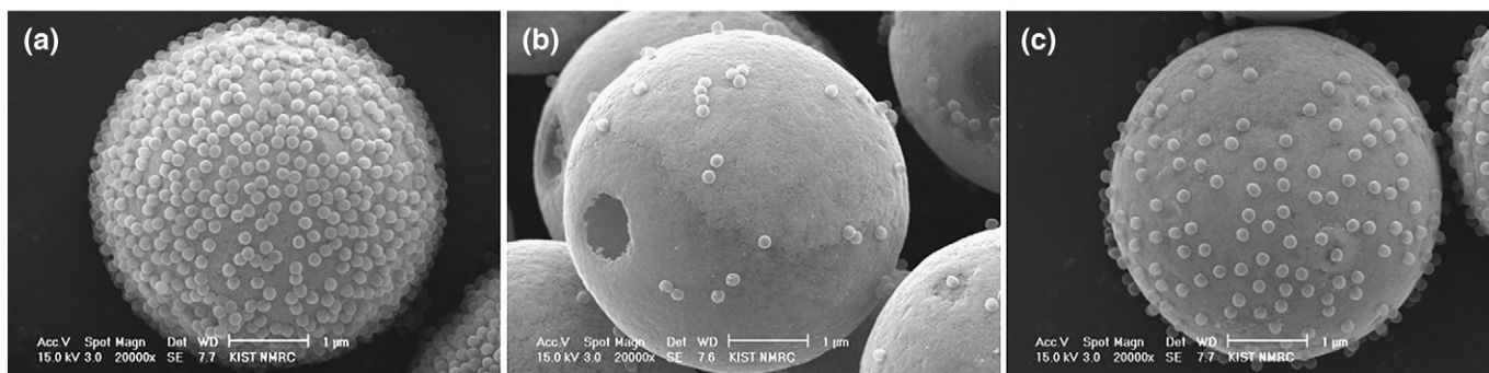
Fig. 3. Morphology of composite particles at various pHs. Each pH is (a) 2, (b) 7, and (c) 11.
