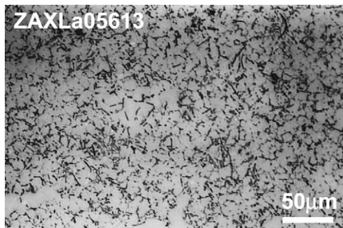
Fig. 3. Microstructure of die-cast specimen of ZAXLa05613 alloy.
