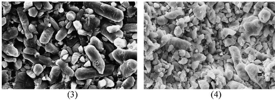
Fig. 3. Representative micrograph of composition B before (3) and after (4) creep tests, at 1350 °C and 300 MPa for 70 h.
