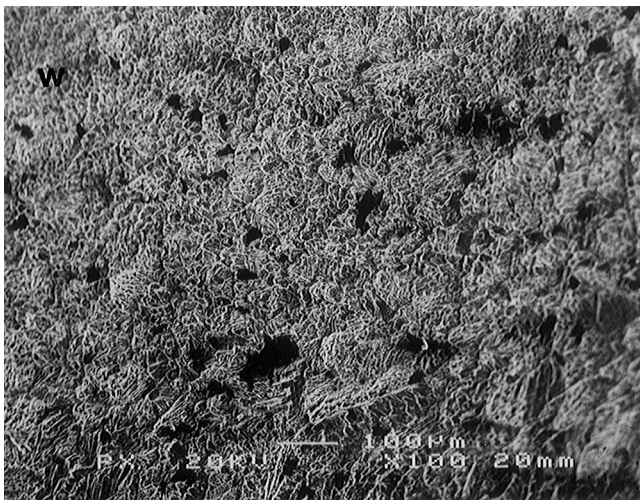
Fig. 17. Sample Code #3, sensitized EB weld (680°C, 1 h). Localized corrosion in the weld. 100×.
