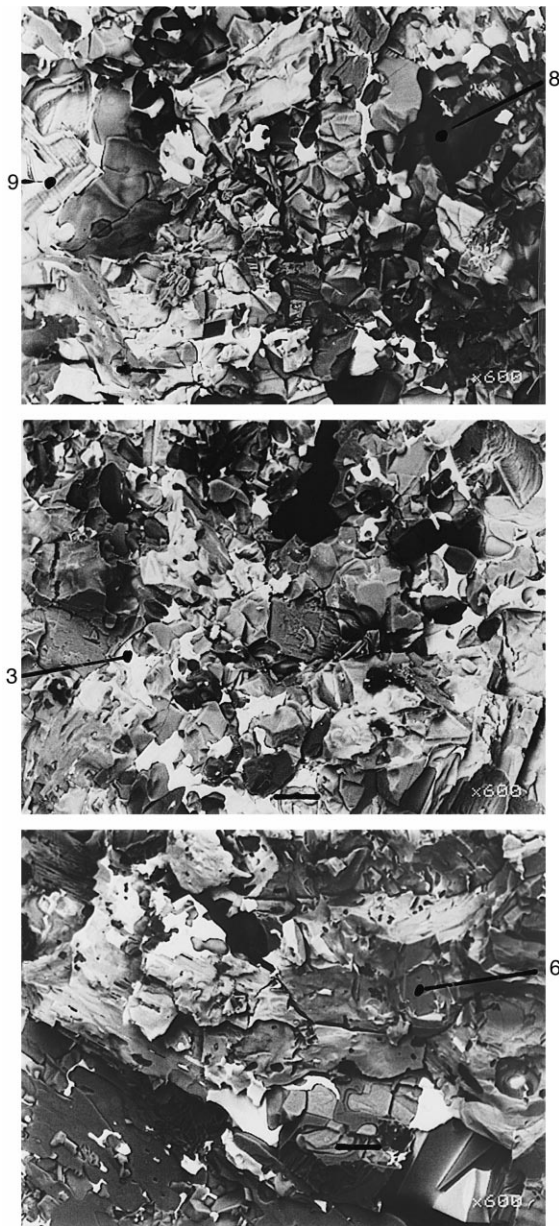
Fig. 3. The SEM micrographs for samples with x = 1.0, 2.2 and 3.0 from top to bottom, respectively. The scale marker is 20 \mu\text{m} .
