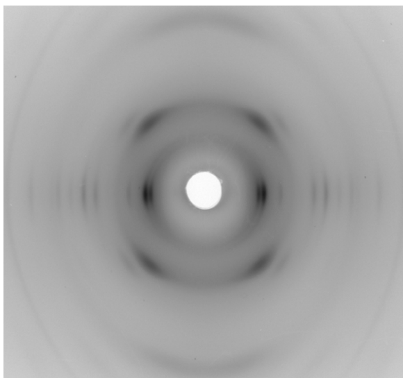
Fig. 2. X-ray fiber spectrum of the 3,4 syndiotactic polyisoprene obtained with (\text{Bipy})_2\text{FeEt}_2\text{-MAO} .
