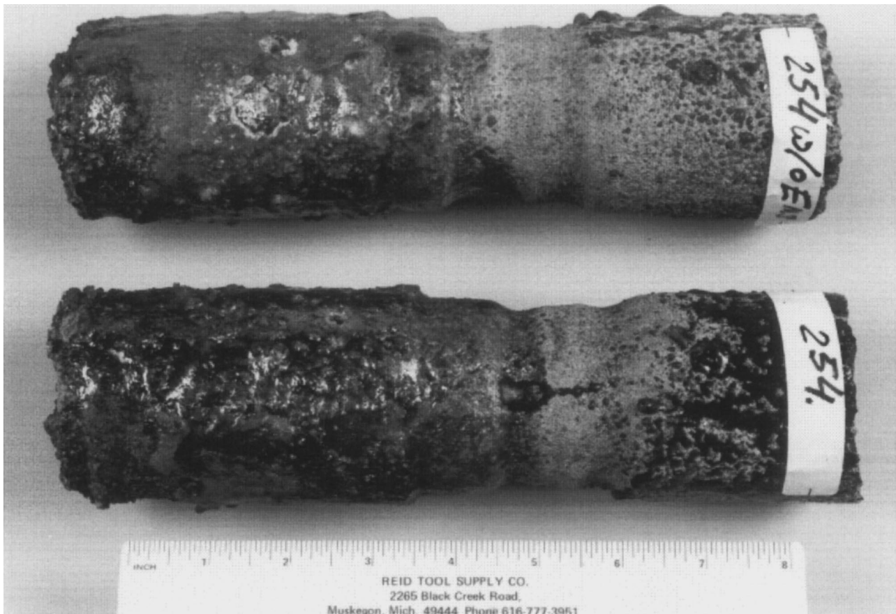
Fig. 14. Erosion of the SEN [12]: (a) without stirring; (b) with dual-coil M-EMS.
