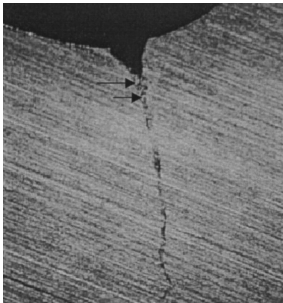
Fig. 6. Longitudinal cracks under chrome chipping with zinc and lead deposits.
