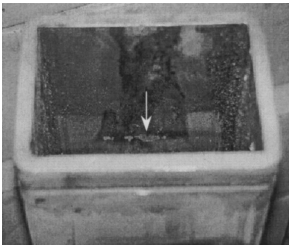
Fig. 5. 5 × 6 3 / 4 " mold tube exhibiting chrome chipping at the meniscus location (arrow).
