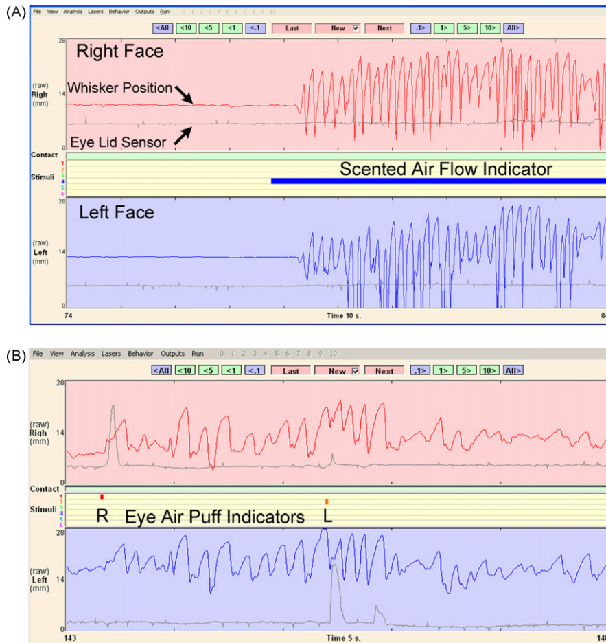
Fig. 5. Whisking and eyelid movement data examples from the acquisition and analysis software's data review screen. (A) Ten seconds of data are shown, with brisk whisking elicited by the presentation of a scented air flow (solid blue bar). The top half (pink background) presents the whisker position (in red) and eye sensor signal (in gray) for the right face, whereas the bottom half (pale blue background) presents the whisker position (in blue) and eye sensor signal (in gray) for the left face. (B). Five seconds of data are shown, with eye blinks elicited by right and left air puffs (see small red and orange markers in the center, respectively). Note how each air puff caused an ipsilateral eye blink, and that bilateral whisking began with the first corneal air puff and continued through the second air puff with only slight alteration.
