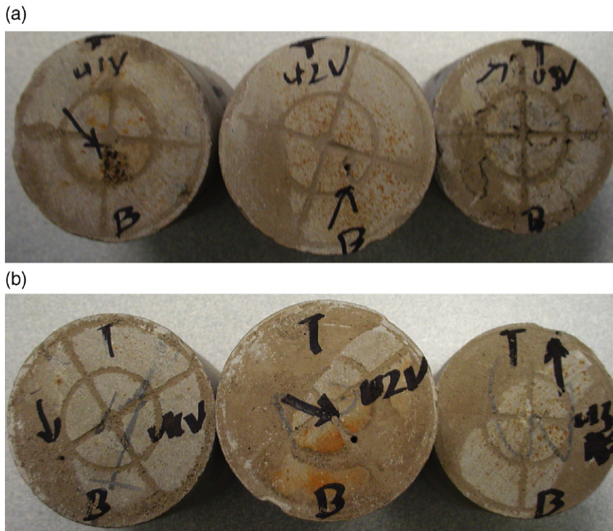
Fig. 14. (a) and (b): Photographs of the three plugs after acidizing showing the actual wormhole sizes at the two ends (injection end at the top, production end at the bottom).
