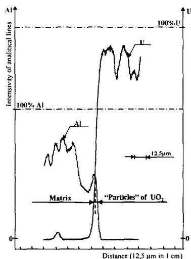
Fig. 1. Distribution of Al and U on the boundary of  $\text{UO}_2$ -matrix after testing at 775 K
