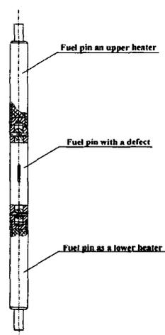
Fig. 2. Sectional fuel pin with an artificial defect
